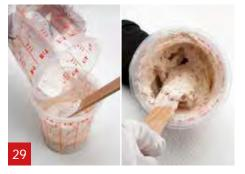
Add as much ATP powder as needed into the A1. Stir firmly till all lumps have disappeared.
