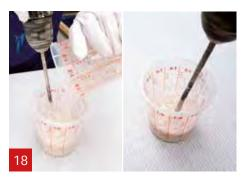
Gently add the A1 powder to the A1 liquid. Stir the mixer till all lumps have disappeared (± 1 min.) resulting in a smooth material.
