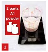
Weigh 2 parts of A1 powder. In this example we use 200 g A1 powder.
