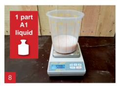
Weigh 1 part of A1 liquid. In this example we use 500 g A1 liquid.
