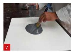
Apply the A1 upon the mould and spread with a brush.
