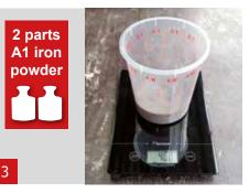
Weigh 2 parts of A1 iron powder. In this example we use 400 g iron powder.
