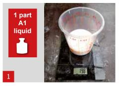
Weigh 1 part of A1 liquid. In this example we use 200 g A1 liquid.
