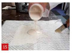
Apply another layer of A1 on the triaxial fibre...
