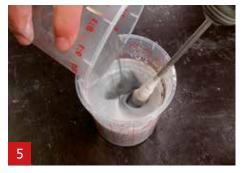
Add the A1 iron powder to the A1 and stir for 1 minute.
