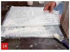
Apply a piece of triaxial fibre with the same size as the object on the surface and smoothen it with a brush from the center.
