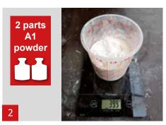
Weigh 2 parts of A1 powder. In this example we use 400 g A1 powder.
