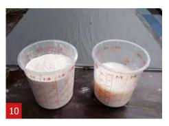
When the panel is dry, weigh 450 g A1 liquid (1 part) and 900 g A1 powder (2 parts).
